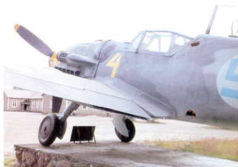
Left. A front view showing such details as the narrow-track undercarriage, wheel wells, segmented spinner and tropical air filter. Right. A close-up of the fuselage showing well the grey camouflage scheme and very carefully applied markings.
