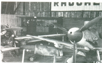
Shown inside this hangar were several Bf 109Fs of JG 52, the one on the right being fitted with underwing gondolas for two 30-mm MK 108 cannon.
