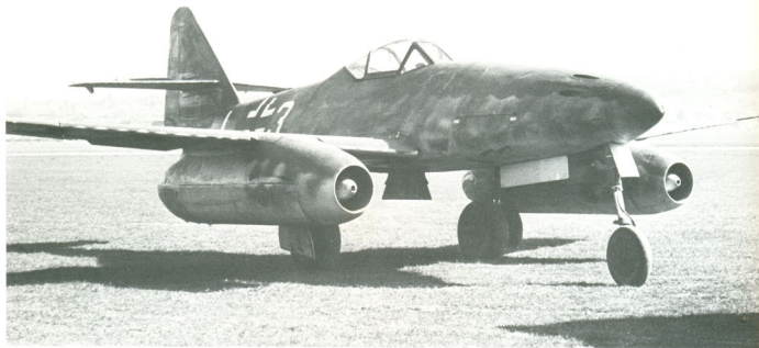
Upper and lower. Zürich-Dübendorf airfield in neutral Switzerland was the recipient of many aircraft from both sides including this 9./JG 7 Me 262A-1b, W Nr 500071, which was flown in on 25th April 1945 by Fr Hans Mutke. A Swiss report described its color scheme as moss green and olive green on top with pale blue undersurfaces. The forward rear fuselage band was red and the rear one, dark blue.
