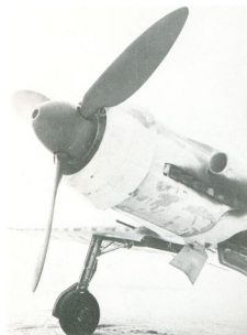
Left. The sleek nose of the Ta 152 V7, W Nr 110007, one of three such aircraft tested during the winter of 1944/45. Its DB 603 engine gave it an outstanding performance. Right. An extremely rare shot of an operational Ta 152H, W Nr 158167, photographed inside a hangar somewhere in Germany.
