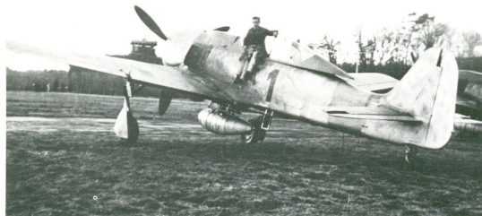
This Fw 190A-7/R2, Black 1 of 2./JG 11, was fitted with two 30-mm MK 108 cannon and was normally flown by either Zwernemann or Doppler.
