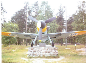
Left. A front view showing such details as the narrow-track undercarriage, wheel wells, segmented spinner and tropical air filter. Right. A close-up of the fuselage showing well the grey camouflage scheme and very carefully applied markings.
