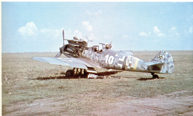
Upper and lower. These two exceptional photographs depict a Bf 109G, White 10, of I./JG 52 being serviced somewhere on the Eastern Front. The lower shot shows particularly good detail of the Daimler-Benz engine and the way the divided cowling panels hinged at the top. Of special interest is the obviously fairly new factory scheme featuring RLM 76 on the upper flying surfaces in conjunction with the same color elsewhere plus liberal blobs of RLM 02, 74, and 75. Even though the yellow rear fuselage band was also fairly new, its pale color is obvious.
