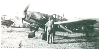
Another variant in the Messerschmitt series was the Bf 109G-6/R2 which was fitted with WfrGr 21 rocket launchers under the wings.
