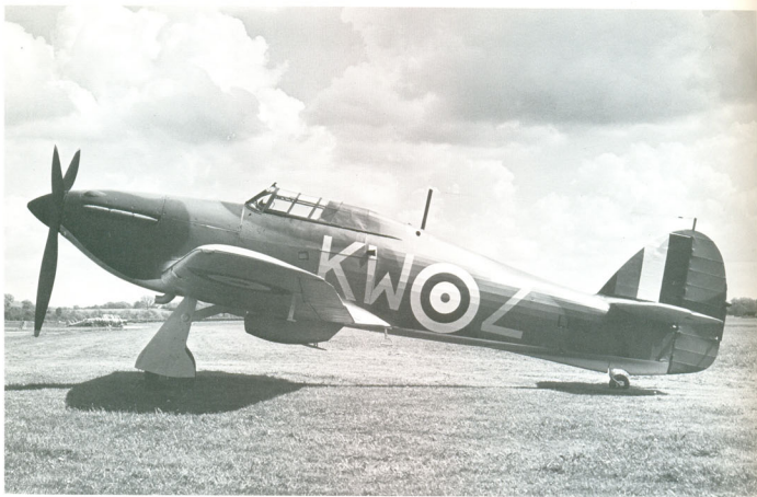
The Hawker Hurricane Mk I, which bore the brunt of the Battle of Britain. An exceptionally strong aircraft which could take tremendous punishment, it was nevertheless at a disadvantage compared to the faster Bf 109E.
